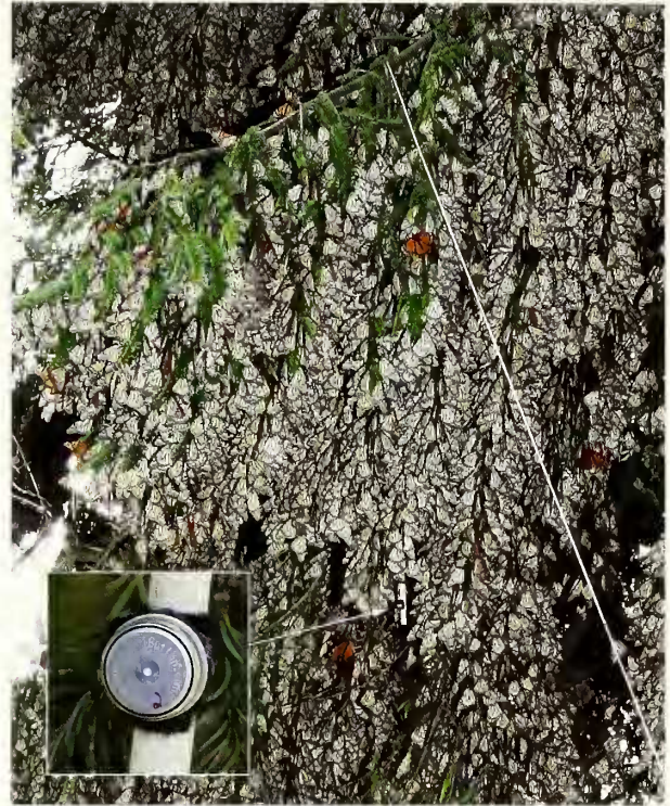
FIG. 5. The experimental dowel inserted into experimental cluster 2 on an oyamel fir bough on 9 Jan 2007. The bottom of the dowel with an exposed hygrochron is evident; the other three hygrochrons are inside the cluster. The inset is a closeup of a hygrochron attached to a dowel with Velcro.
